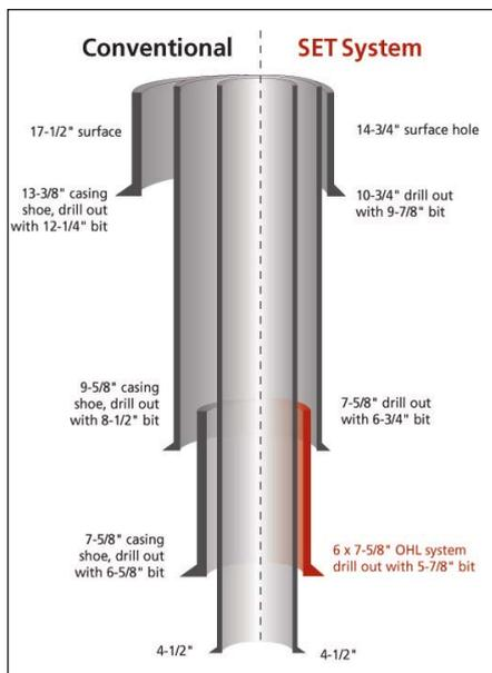
*By incorporating solid expandable technology into the wellbore design, the operator reduced overall drilling time by 21 days. Additional savings were realized when swellable elastomer technology was used with the expandable system to provide zonal isolation — eliminating the need to cement. (Images courtesy of Enventure Global Technology)*
