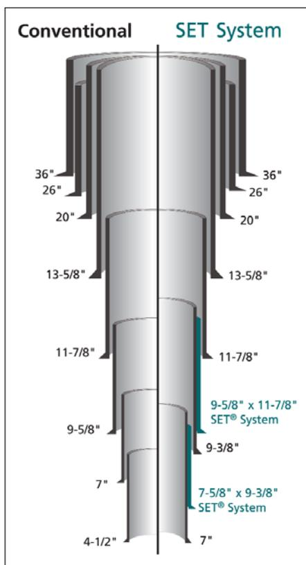
*In the Gulf of Mexico shelf, an operator used two expandable systems to reduce drilling time from 200 days per well to 60 to 90 days per well.*
