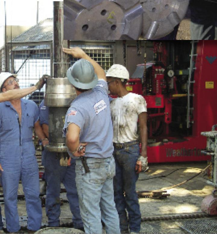
grade pipe right now, which is 80,000 psi yield strength steel. After it is expanded, the yield strength is more than 90,000 psi."
