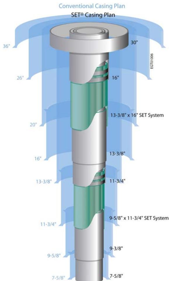
**Figure 5 – Solid expandable tubular technology used in the well drilling industry. Expanding pipe sections at extended depths avoids loss of diameter as depth increases.**
