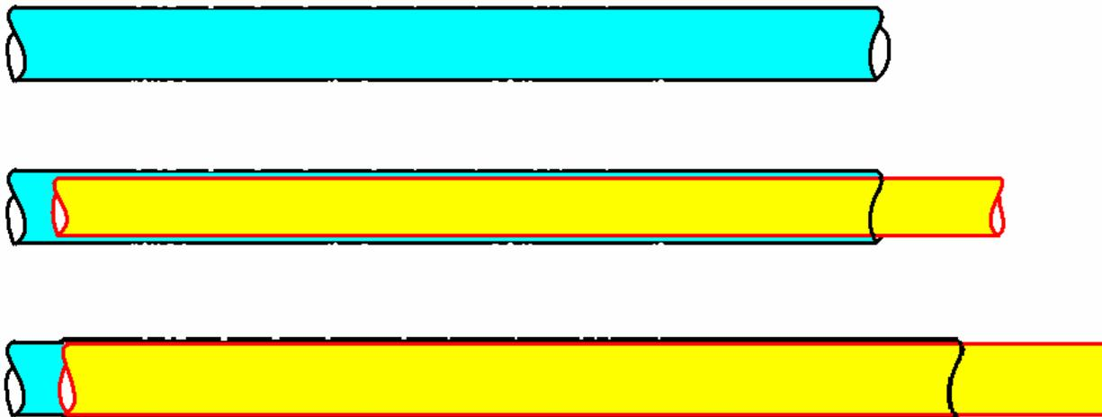
**Figure 6 – Conceptual drawing of how solid expandable tubular technology would be applied to the pipeline industry. This figure illustrates the existing pipe (top), the new pipe inserted in the old pipe (middle), and the expanded new and old (bottom).**
