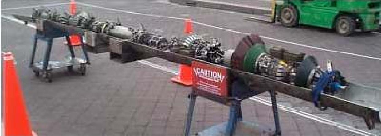
**Figure 2 – Smart pigs are typically used to inspect high pressure pipelines.**
