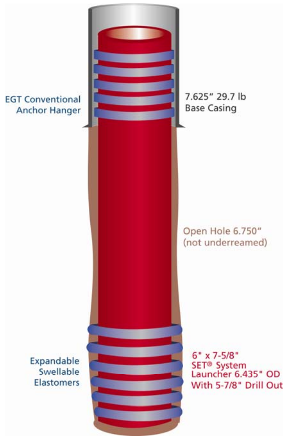
Figure 1: Solid expandable technology enables slimmer well design while using swellable elastomers and eliminating underreaming operations.
