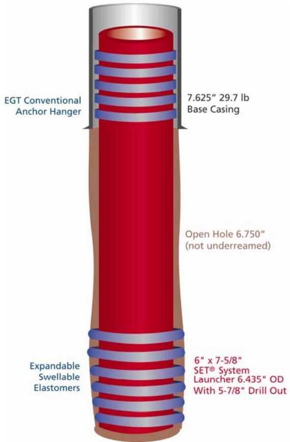
Figure 1: Solid expandable technology enables slimmer well design while using swellable elastomers and eliminating underreaming operations.
